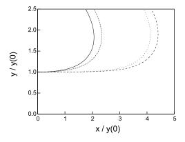
**Figure 3.** A comparison of the compacted and uncompacted normalized Ernst profiles in two different cases: (\_\_\_\_\_), compacted profile, r = 1; (\_\_\_\_\_), uncompacted profile, r = 1; (...,), compacted profile, r = 3; and
